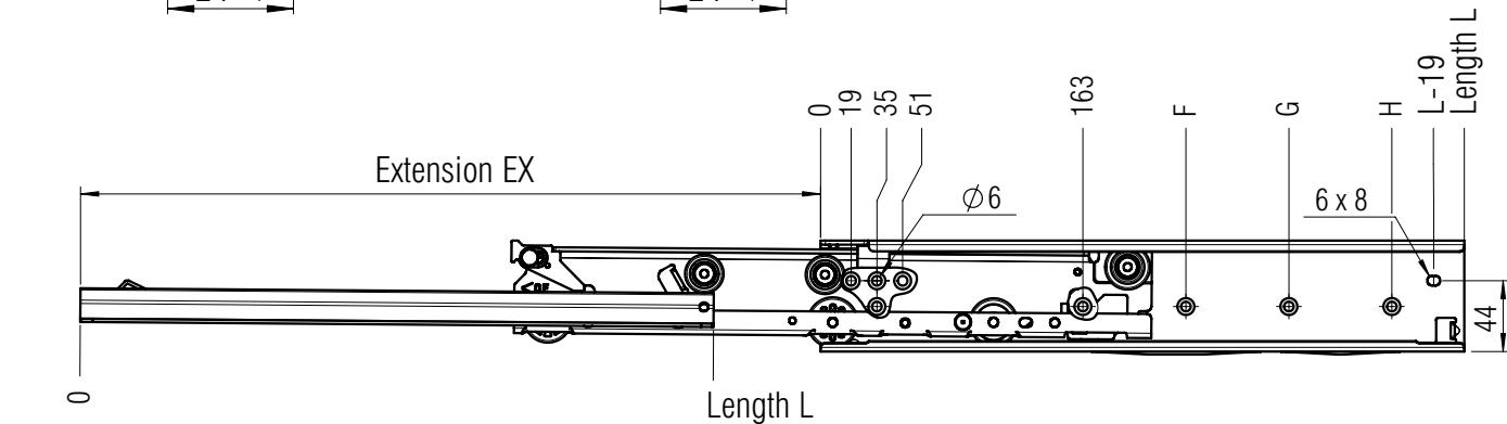
screw holes for 4,5 mm spax screws
