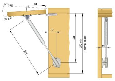
The dimensions of the above drilling plan refer to carcases which use standard sprung hinges and mounting plates 0mm
