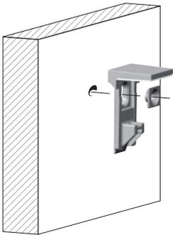
Recommended fixing countersunk screw type - head Ø 5 mm max.
