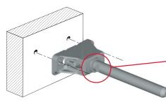
**VERY IMPORTANT** Triade Maxi has to be installed with the arrow facing upwards.
