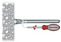
SHELF INSERTING AND LATERAL ADJUSTMENT
