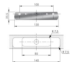
VERY IMPORTANT Centre of the hole is shifted 3,5 mm upwards. Please keep in mind when levelling the shelf.
