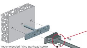
VERY IMPORTANT Triade has to be installed with the writing "TOP - ALTO" facing upwards.
